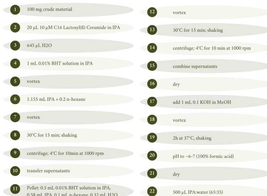
FIGURE 2.2: Workflow of the final two-step liquid-liquid extraction method used for GIPC sample preparation.
