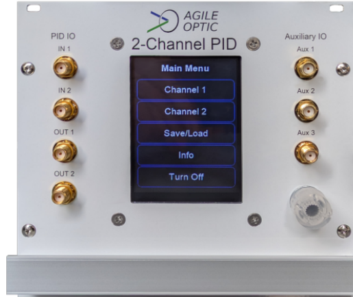
Figure 3.20.: PID main interface, which allows to input the error signal from two distinct cavities 'IN 1/2'. After processing the information, a feedback 'OUT 1/2' is returned to the individual piezo mirrors for length stabilization of the resonators. The auxiliary outputs 'AUX 1/2' are used for power monitoring. 'AUX 3' is optional and internally not connected.
