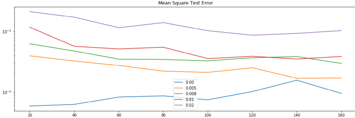
Figure 4.5: Mean squared errors of the approximation to the inverse problem of the Euler-Bernoulli equation on the test set for five different noise levels: 0.00, 0.005, 0.008, 0.01, 0.02. The x -axis shows the ambient dimension which corresponds to the number of measurements D , the y -axis records the mean squared error of the reconstruction over the test set.
