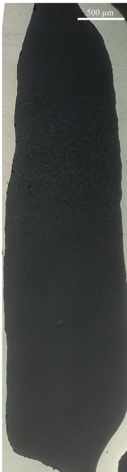
S7. Fig.7. Reflected light microscope image of Sample 1150d-Cr-doped-5min. To note the size gradient inside the sample and the lack of Cpx grains (<5% of the area) in the hottest portion of the sample, probably at T > 1170^{\circ}\text{C} .
