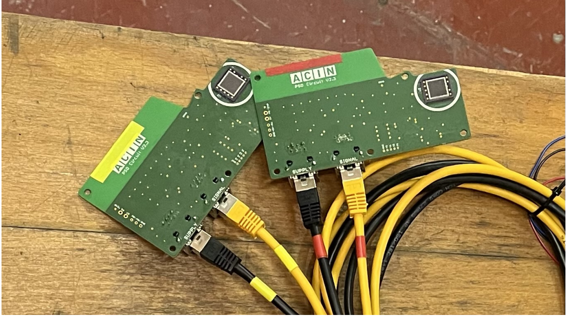
Figure 2.3.: Photograph showing the second iteration of the PSD circuits as it was used at the telescope, including marked Ethernet connections for power (black) and signal (yellow).
