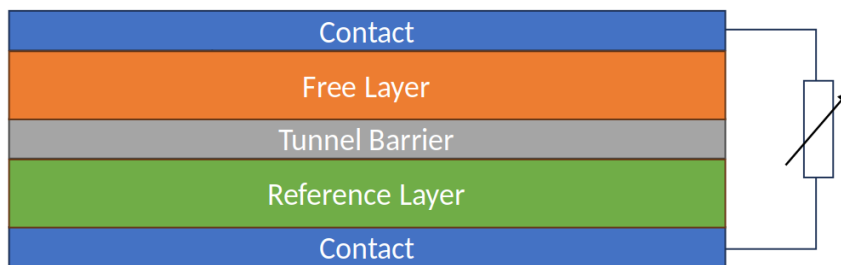
FIGURE 2.1: Schematic structure of a Tunnel Magnetoresistance (TMR) sensor. The device consists of a Free Layer, Tunnel Barrier, and Reference Layer, sandwiched between Contact electrodes. The magnetization of the Free Layer is variable, whereas the Reference Layer maintains a fixed magnetization, enabling resistance changes based on their relative alignment.
