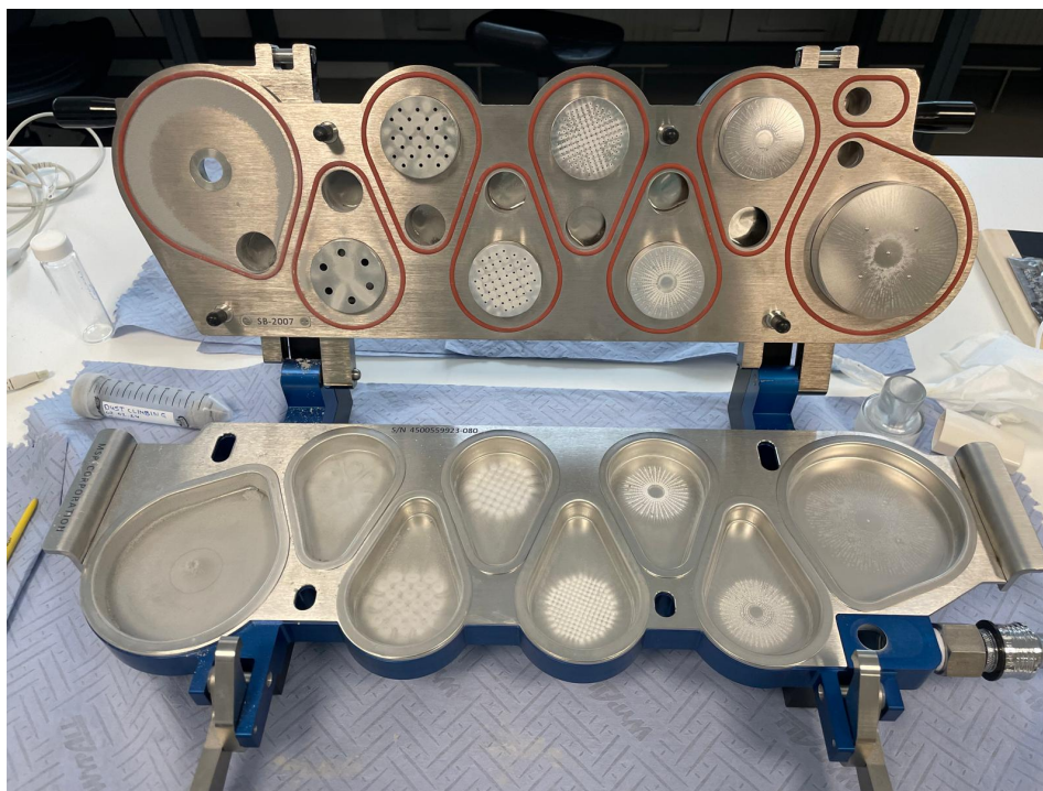
Figure 3.1.: Next Generation Pharmaceutical Impactor for Dust Size Separation. Trays 1-8 from left to right.
