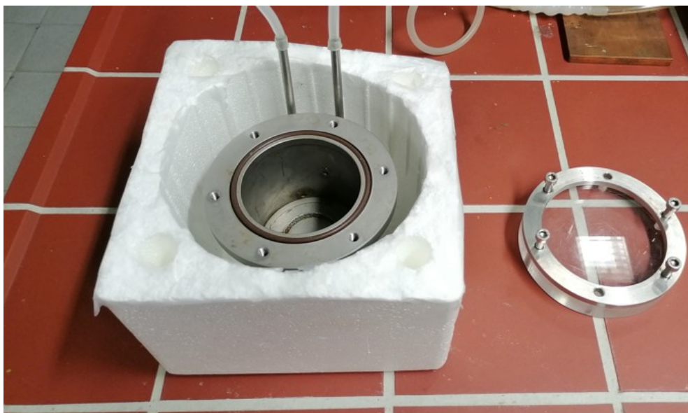
Figure 3: Apparatus for cryogenic loading of Argon. Left: Styrofoam container, used for placing the autoclave (middle) inside and filling the container with liquid nitrogen in the space between to cool down the gaseous Ar inside the autoclave. Right: lid for the autoclave.
