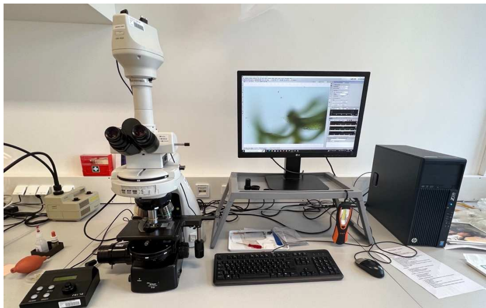
Fig. 15. Light,- and epifluorescence microscope Nikon Eclipse NI and NIS Elements Software.
