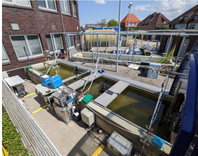
Figure 1. The Sea Surface Facility (SURF) at ICBM Wilhelmshaven, Germany includes a basin, a retractable roof, and several on-site instruments to control some water parameters and to monitor the physical parameters (see text for a detailed description).
