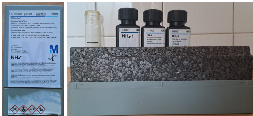
Figure 9 The determination kit for the ammonium content from Merck KGaA (left); the test tube and the three reagents are shown at right
