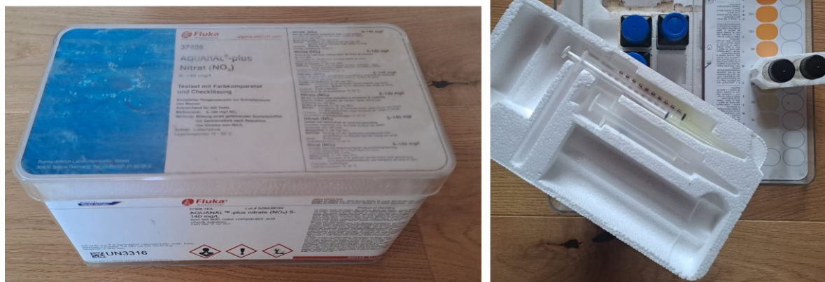
Figure 10 The Fluka Analytical Aquanal-plus nitrate determination kit (left). The sample glasses, the reagents (black containers) and the colour scale for comparison is shown at right
