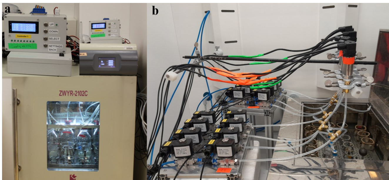
Figure S3: Images of the experimental setup of the GPC. a. The gas lines are introduced into the air incubator from the side and attached to the bottles. The controlling system for data monitoring and power supply is additionally shown. b. GPC set-up in the fume hood.
