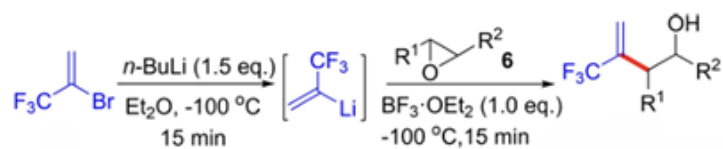
Scheme 18. \text{BF}_3 -promoted ring-opening reactions of BTP with oxiranes
