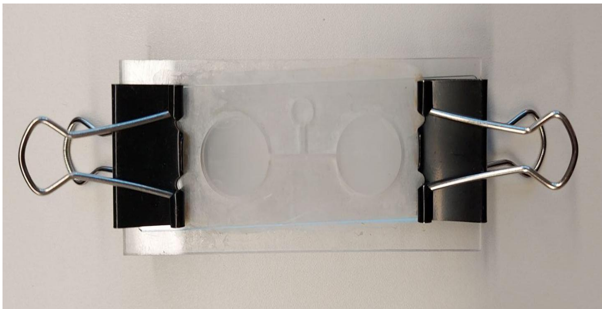
Figure 23. T-shaped choice arrangement (© Mustafa Altintas).
