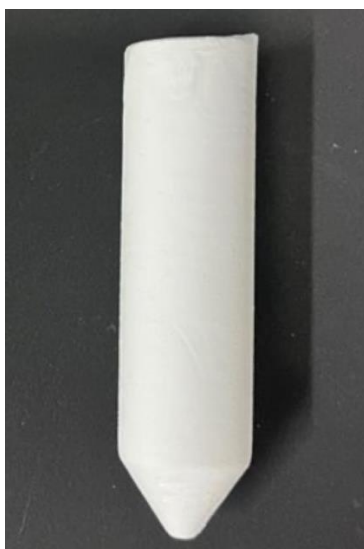
Figure 13 - polyHIPE stabilized by as-synthesised P(AAm- co-4St)
