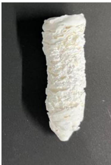
Figure 14 – polyHIPE stabilized by 0.73 wt % PVA and 6.38 wt % Triton X-405, as described by Kulygin and Silverstein 42
