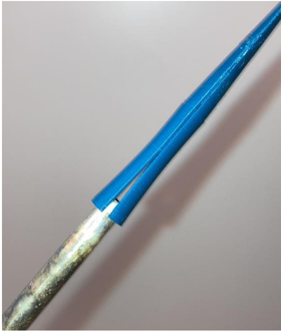
Figure 9. This figure shows the damage that was created when inserting the mouthpiece onto the bocal, and the air leakage that needed solving.
