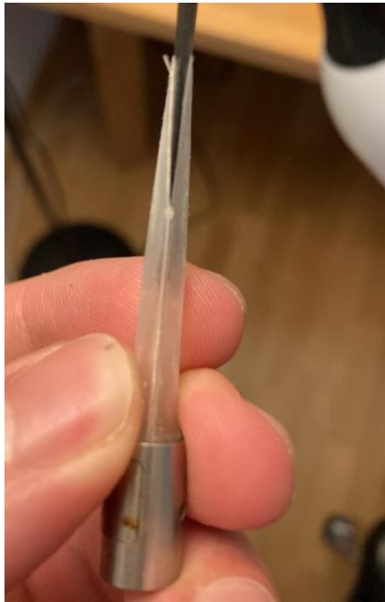
Figure 11. In this figure our player is using one of his reed-shaping tools to show how his “medium-hard Bassoon reed” made by the company Légère isn’t glued completely. The distance between the entrance of the reed and the point where the two reeds were glued together is 15mm.
