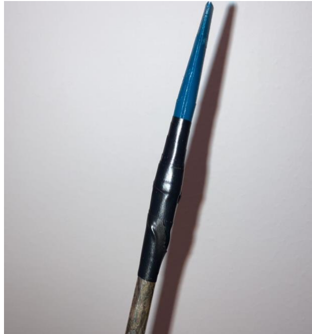
Figure 10. This figure shows our solution of taping the mouthpiece to the bocal to avoid air leakage and further fracturing.
