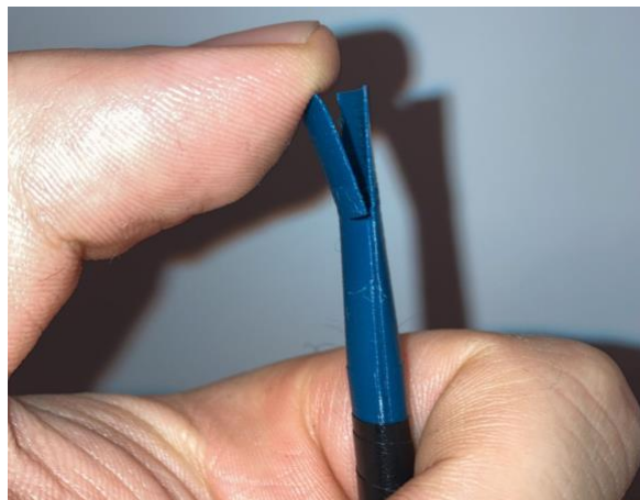
Figure 13. This figure shows broken 3D mouthpiece, that broke during recording the Fourth register of our 15mm “cut in depth” on both sides at 12,5mm from the mouthpiece entrance.
