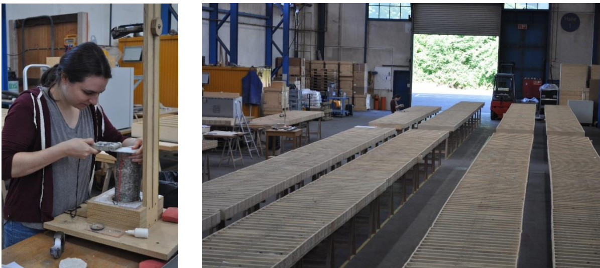
Fig. 8: Left: Measurements of core structures with a geological compass. The core was oriented according to core orientation lines in the goniometer. Right: Laid-out cores in the Nagra core storage facility Würenlingen.
