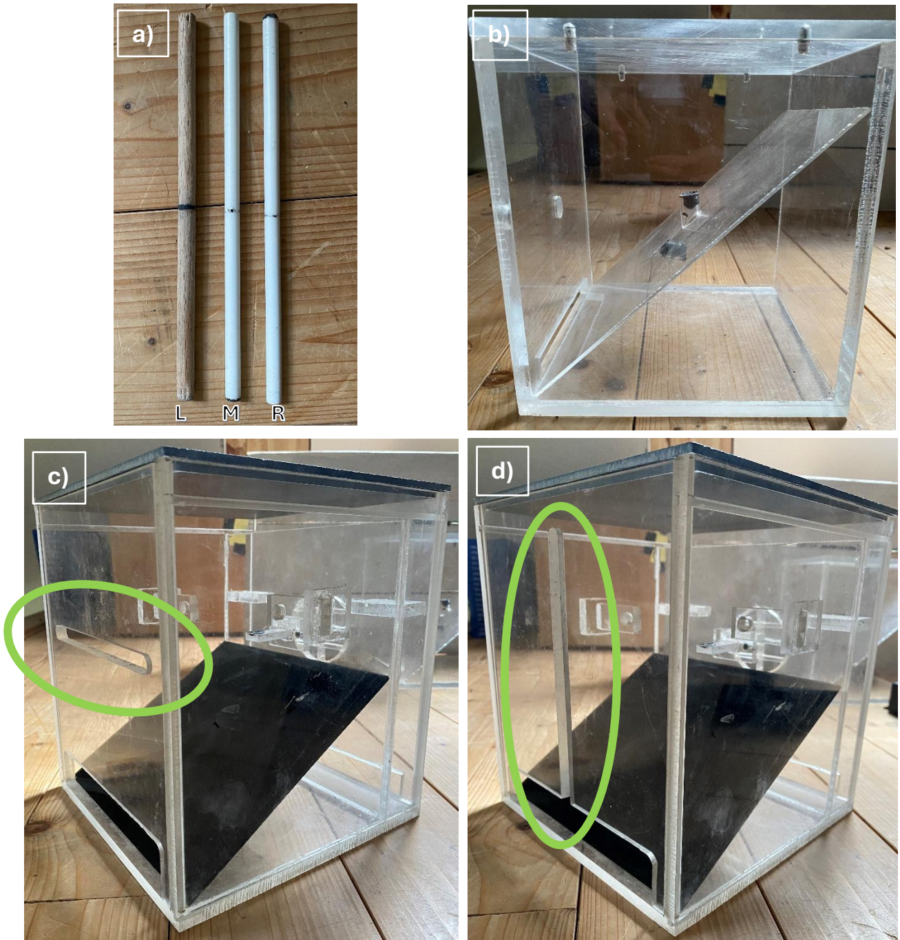
Figure 1: Apparatuses and tools used in the experiments. (a) Tools used in both experiments: Left (L): a light wooden stick, 17.5 cm in length, uniformly balanced, marked in the middle, and used for the Base Technique experiment with box (b). Middle (M) and Right (R): unbalanced sticks used in the unbalanced test (Box c) and d)) made from hollow, sturdy plastic tubes with a 12 g weight inside the lower third. Both sticks are physically identical except for the markings: (M) has the light side marked, and (R) has the heavy side marked. (b) Base Technique apparatus: a transparent Plexiglas box with a slide inside and a central stand for the reward, featuring two front openings: a central circular hole for tool insertion and a lower slit for reward retrieval. (c) and (d): Apparatuses for the unbalanced test: identical boxes differing only in the front window design, with (c) having a horizontal opening and (d) a vertical opening. Both apparatuses feature a reward stand mounted on the back wall and a black Plexiglas slide inside, designed to facilitate the sliding of the reward down to the retrieval slit at the bottom.
