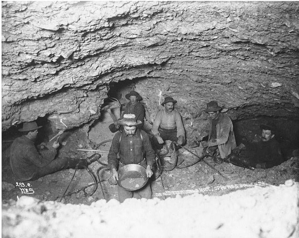
Figure 21: Miners thawing frozen ground with steam in an underground gold mine lit by candlelight, Gold Hill, probably 1898; Photograph: HEG232, Eric A. Hegg Photographs, Special Collections, University of Washington Libraries. Courtesy of the University of Washington Libraries.
