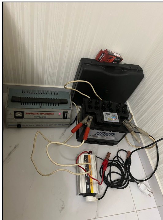
Figure 3. Setup of an Autonomous Energy Supply System Using a Car Battery and Inverter
