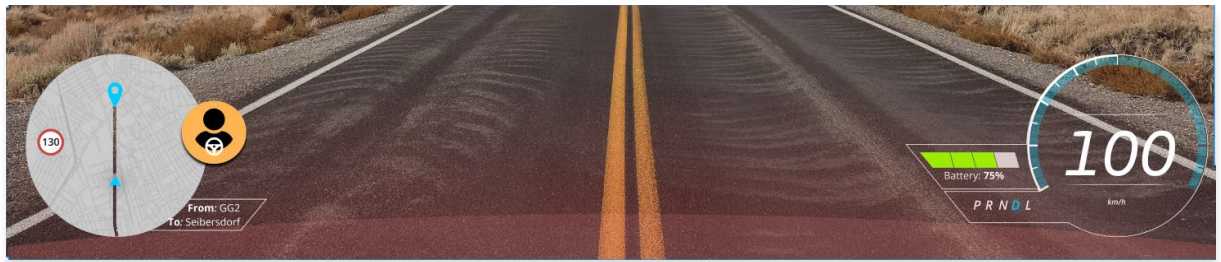
Figure 4 Close-up of the heads-up display during manual driving during a takeover request: A red tint at the bottom of the screen served to draw attention to the heads-up display.
