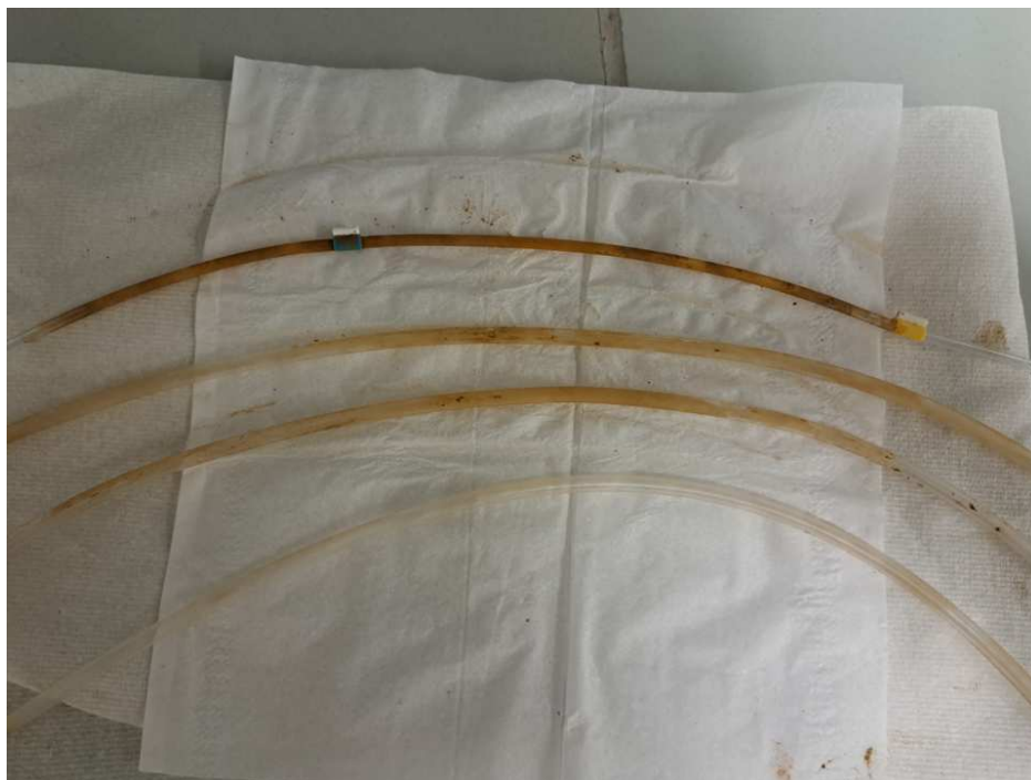
Figure A.6: Artificial roots after being submerged in anoxic soil for 14, 9, 4 and 2 days (from top to bottom) with the tube on the top being peristaltic, the others are silicon tubes, with visible reddish iron plaque
