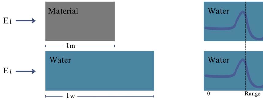
Figure 3.1.: Schematic illustration of the concept of WET [52].
