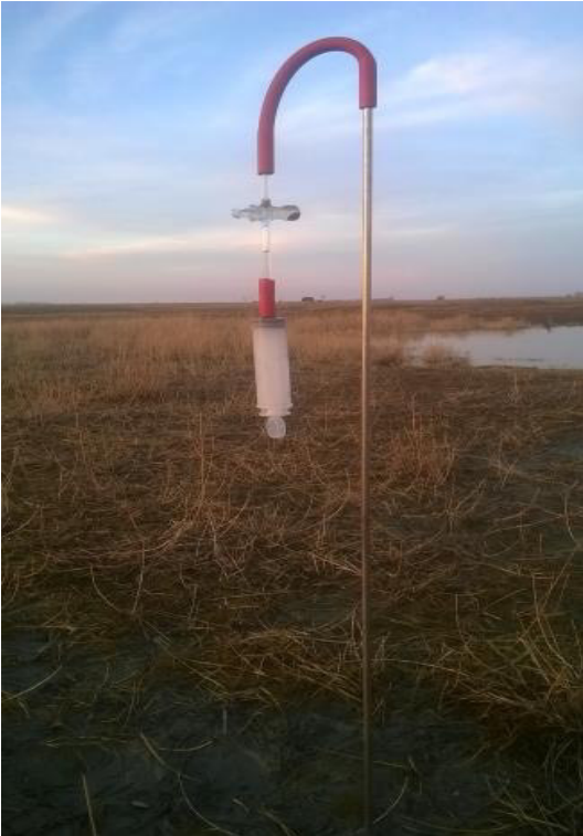
Picture 5: Vacuum pore water collector
