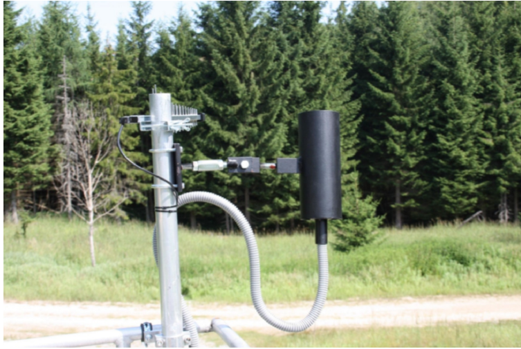
Figure 2.3: In Upper Austria, the 23 Sky Quality Meters (SQMs) are protected by durable black-coated iron cylinders, replacing the typical plastic enclosures. These housings feature multiple sharp spikes on top to deter birds from perching and soiling the equipment. The region has deployed only SQM-LE models, which come with built-in ethernet connectivity. Source: Posch et al. (2018). Reprinted with permission.
