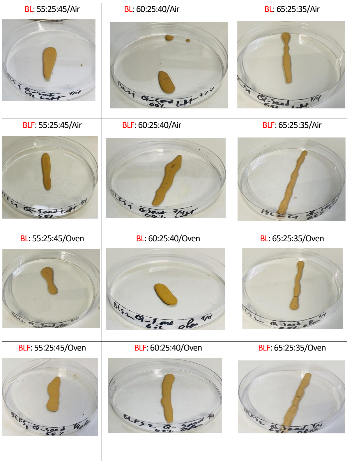
Figure 24: Photographs of ejected and dried BL and BLF formulations at 55 to 65 % solids and 25% Q-sand levels in the solid phase. BL/BLF: sand in water at room temperature 25 °C and oven 70 °C.
