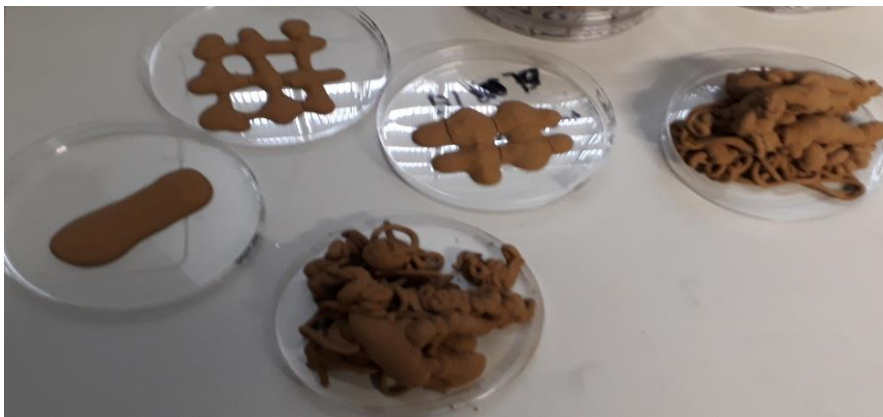
Figure 14: 80% solids content pneumatically sprayed, and dried strands (¼ BL und ¼ S-sand).
