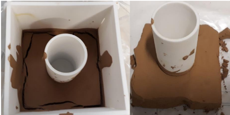
Figure 15: Thick-walled bricks casted from 80% solids content formulations ( \frac{3}{4} BL und \frac{1}{4} S-sand).
