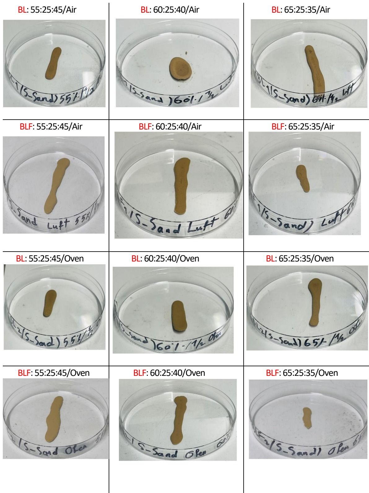
Figure 27: Photographs of ejected and dried BL and BLF formulations at 55 to 65 % solids and 1/2 S-sand levels in the solid phase. BL/BLF: sand in water at room temperature 25°C and oven 70°C.
