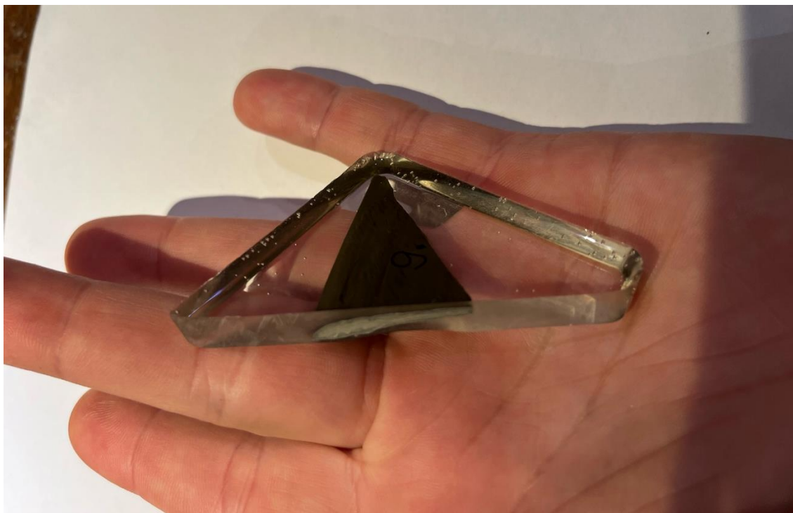
Fig. 28b: Sample AW9 after bedding in synthetic resin
