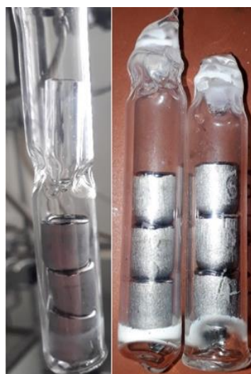
Figure 54 Top: Schematic of the encapsulation process. 1...H 2 /O 2 -torch, 2...quartz glass tube, 3...vacuum rotary vane pump, 4...sealed Ta-crucibles, 5...Ta-spacer. Modeled with CorelDraw 2018. Bottom, left: quartz glass tube filled with 3 closed Ta-crucibles before sealing of the tube. Bottom, right: 2 sealed quartz glass ampoules filled with samples in closed Ta-crucibles.
