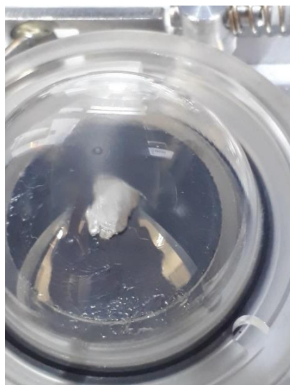
Figure 76 Soft and ductile sample, flattened for XRD investigation.
