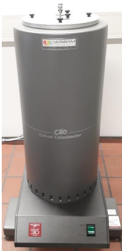
Figure 60 Heat flow 3D-DSC - C80 Calvet calorimeter of Seteram.
