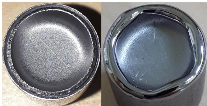
Figure 52 Left: Birdseye view of the closed Ta-crucible before TIG-welding. Right: Birdseye view of the closed Ta-crucible after TIG-welding.
