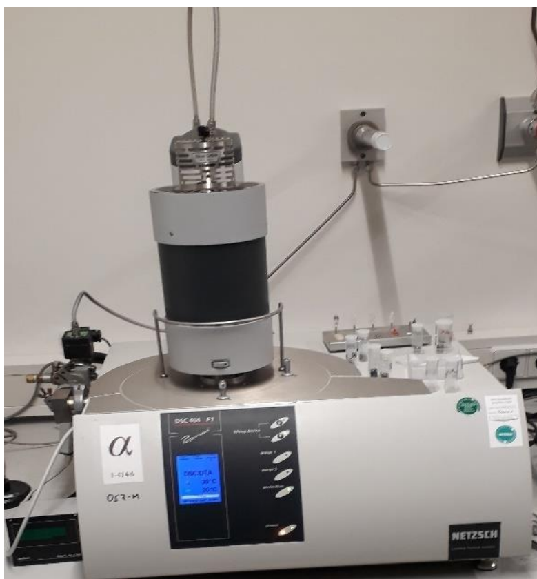
Figure 57 DSC 404 F1 of Netzsch with SiC-furnace used for DTA measurements.
