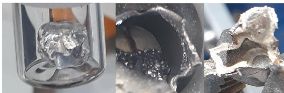
Figure 73 Typical appearance of In-Li alloys in relation to an increasing amount of Li from left to right. In-Li 33 (left), In-Li 9 (middle) and In-Li 14 (right).
