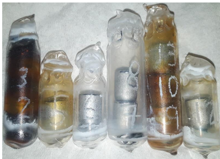
Figure 72 Left- and right-side: Brown to silver-black colored quartz glass ampoules with the samples In- Li 2, 3, 5, 9, 10, 13 and 12. In the middle: Clear quartz glass ampoules with the samples In- Li 6, 7 and 8 for comparison.
