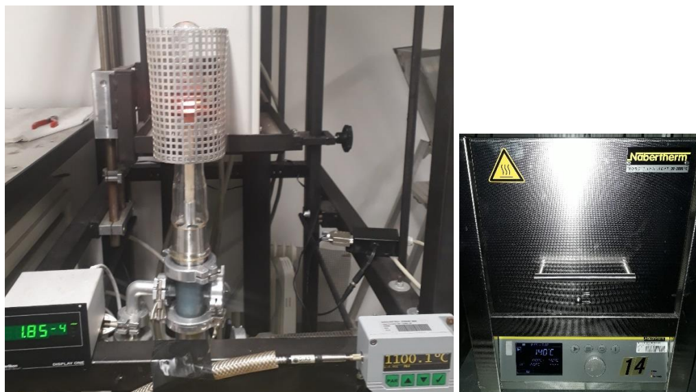
Figure 55 Left: Induction furnace. The display in the left corner shows the pressure in mbar, the display in the right corner shows the temperature of the crucible. Right: Muffle furnace of Nabertherm.
