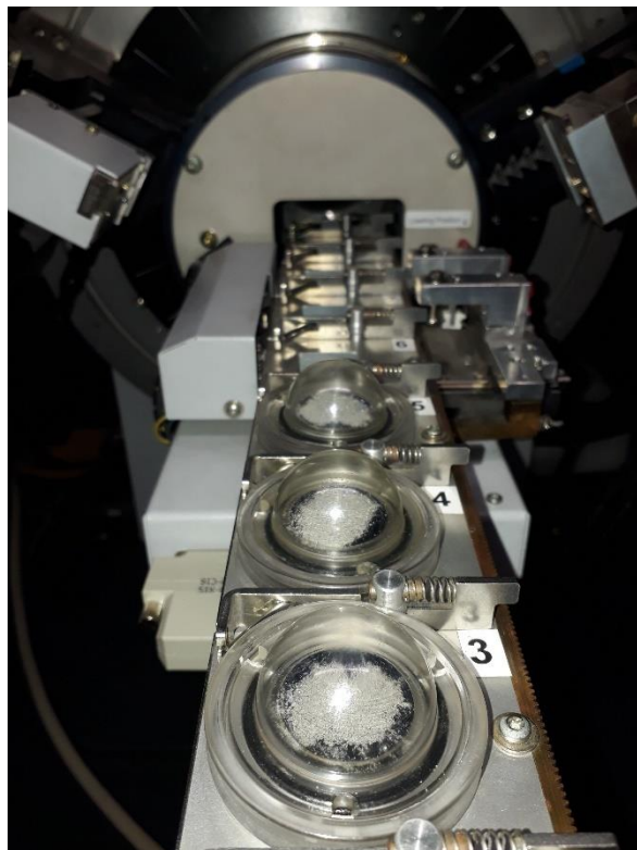
Figure 64 “Old” Bruker D8 Advance Diffractometer. Left: X-Ray tube. Middle: Autosampler loaded with 3 sample holders with dome, containing powdered In-Li samples under dry Ar. Right: 1D-detector.
