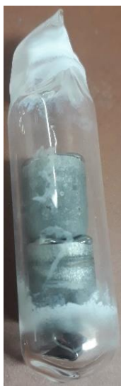
Figure 63 Annealed and quenched sample In-Li 3 (upper crucible) and In-Li 4 (lower crucible) in quartz glass ampule.
