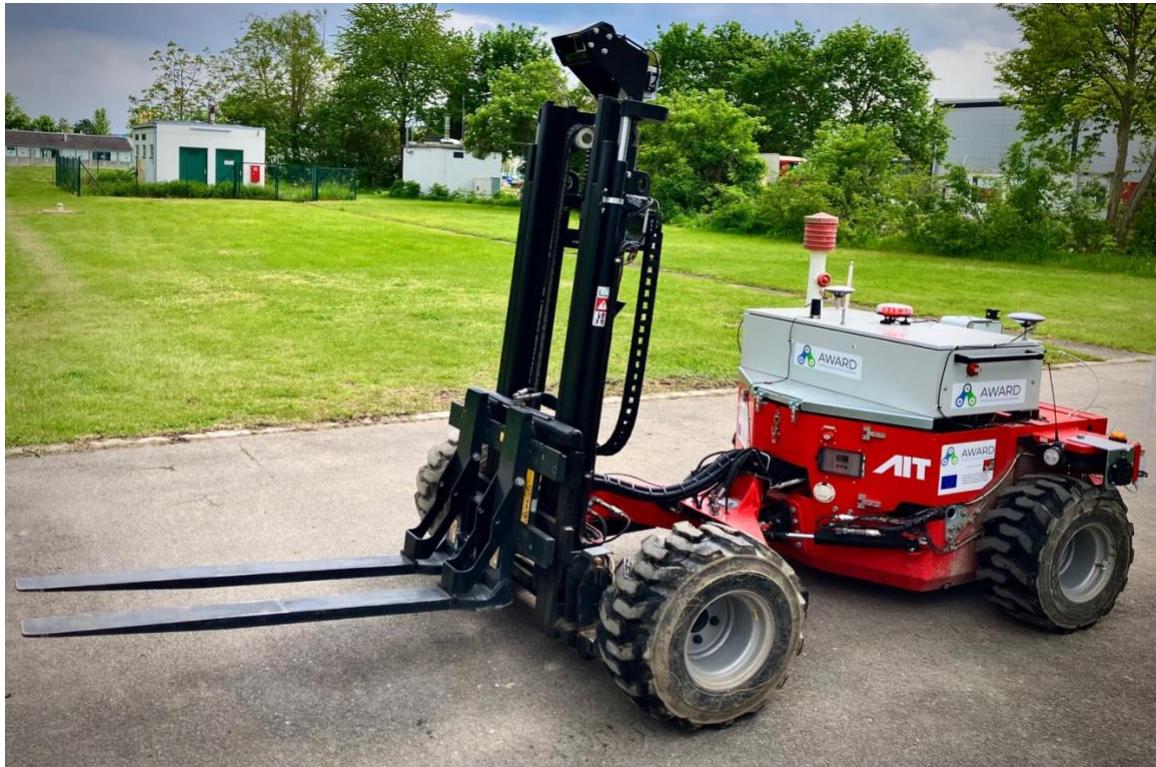
Figure 21: The modified forklift truck Crayler by the team of the AIT.
