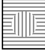
Figure 3.3.: Grating layout of an SLM region: The pupil in the centre has a grating diffracting an incoming beam horizontally. The light outside of the circular pupil is diffracted upwards by a vertical grating.
