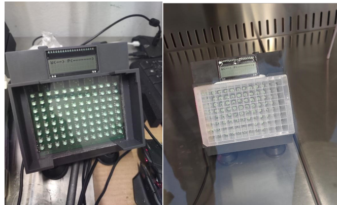
Figure 5.3: Sortinator device with (right) and without (left) a 96 well plate
