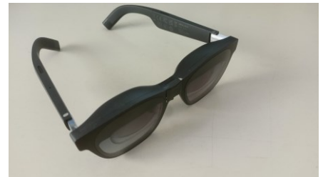
Abbildung 8: See-Through-HMD/ Smart-Glass: XREAL Air2
