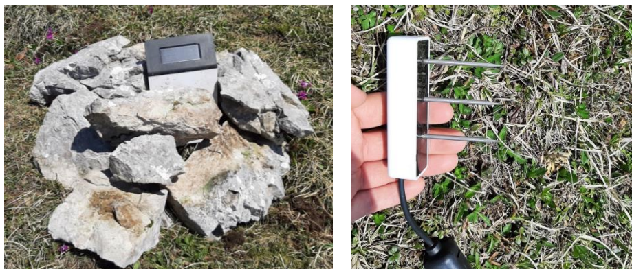
Fig. 16: Left: ZL6 data logger with an integrated solar charging panel, stabilized with rocks; Right: Teros 12 sensor for measuring volumetric water content.
