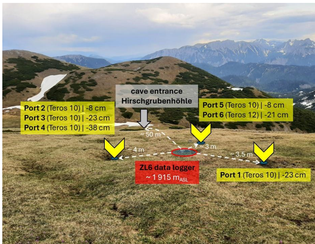
Fig. 17: Overview of the setup for measuring volumetric soil water content in the supposed catchment area of the cave drip water. Yellow arrows indicate locations of sensors, differentiated with associated values of depth below the surface. The ZL6 logger (red) is located at approximately 1915 m ASL and 50 m from the cave entrance. Direction of view is roughly South.
