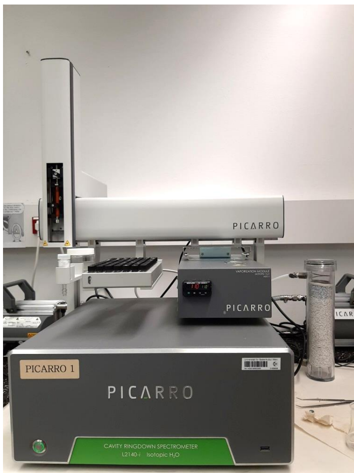
Fig. 21: Picarro TM L2140-i isotopic water analyzer with CRDS technology.
