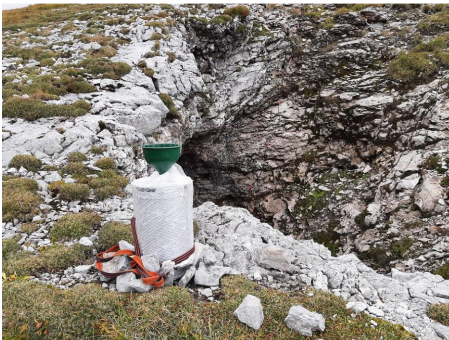
Fig. 18: Rain sampler at the entrance of the Hirschgrubenhöhle.
