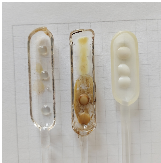
Figure 33: Glass crucibles showing the final results after three consecutive reheatings: the leftmost shows the commodity cPET sample when using nitrogen, the middle one the commodity (top) and high purity samples (bottom) under air and the rightmost the high purity PET pellets under nitrogen gas. For reference, the background grid is 5 mm in width.
