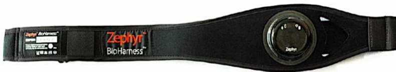
Figure 3. BioHarness 3 Sensor chest belt (Biopac Systems Inc., 2015).
