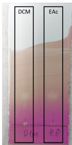
Figure 54: TLC for solubility comparison between either \text{CH}_2\text{Cl}_2 (DCM) or ethyl acetate (EAc) mixed 1:1 with petrolether. Staining was done via \text{KMnO}_4 dip with subsequent heat gun treatment.
