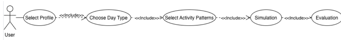
Figure 3.4.: Use case diagram of the system's general workflow
