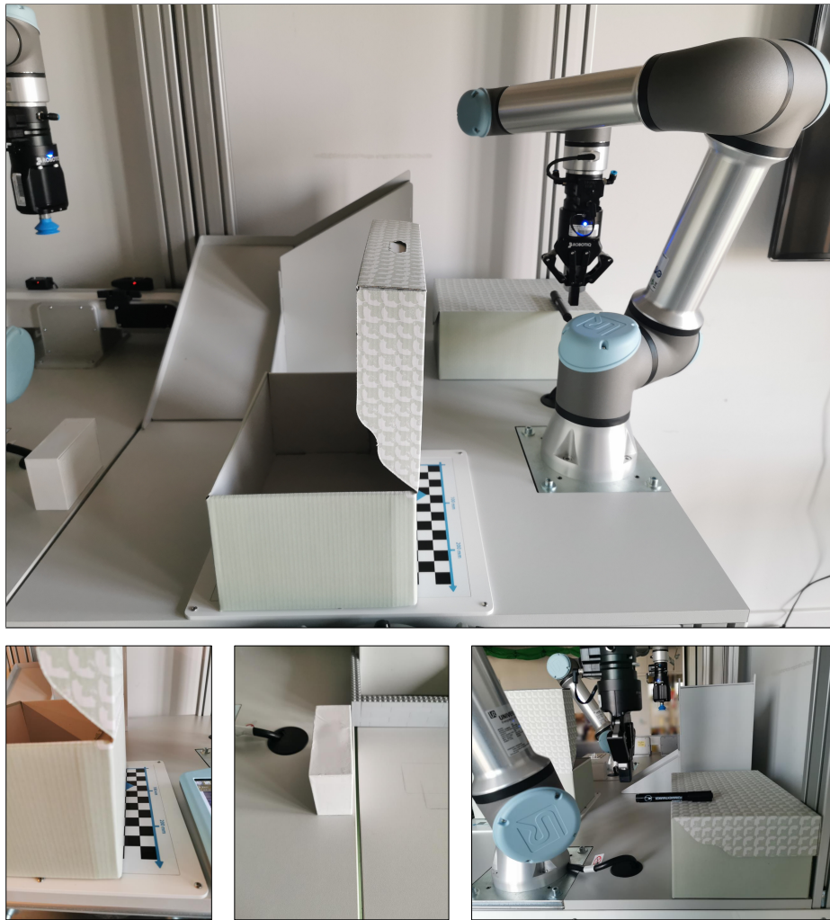
Figure 7.11: Physical cobot cell setup for Scenario 2: Pack-and-Paint
