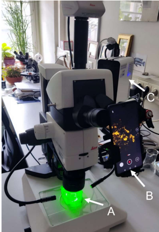
Figure 4 | Experimental setup. Sample A was placed under the stereomicroscope, exposed to green light from the CoolLED system C and captured by the camera B.
