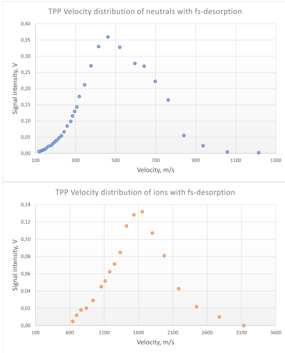
Figure 5.8: Measured velocity distributions for ions and neutrals of TPP. Neutrals were desorbed with 343 nm wavelength, 290 fs repetition rate and E_P \approx 10 \mu\text{J} pulse energy focused to the wheel with a fluence of F = 4.68 \text{ mJ/cm}^2 . The \text{F}_2 laser postionized the particles with 157 nm wavelength and 1.58 mJ pulse energy. Ions were desorbed with a different pulse energy of E_P \approx 15 \mu\text{J} and focus, with a fluence of F = 4.81 \text{ mJ/cm}^2 .
