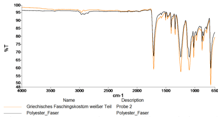
Figure 63: Spectrum greek costume white part (polyester fiber).
