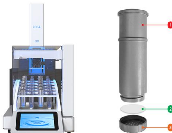
Figure 18: CEM EDGE extraction apparatus and Q-Cup (1), Filter (2) and threaded bottom (3). (C.E.M. Corporation 2017)
