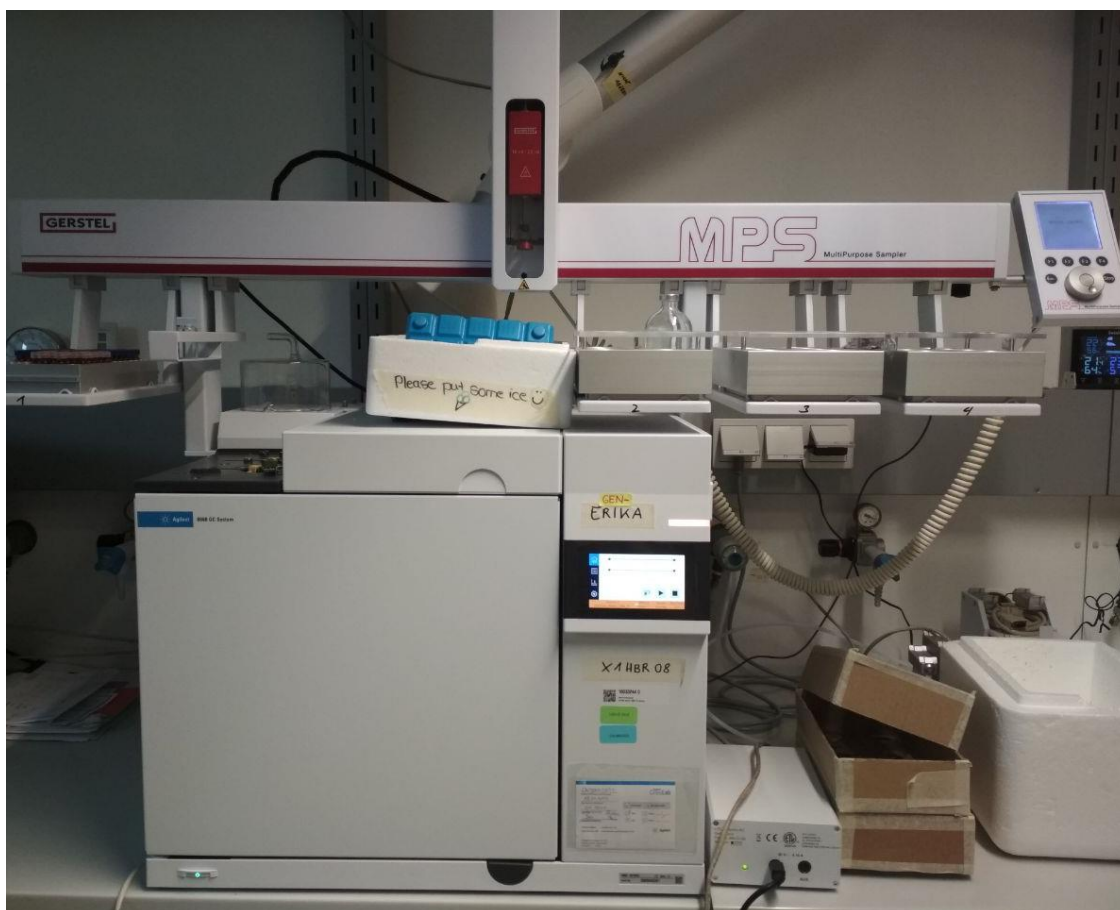
Fig. 20: Gas chromatograph Agilent 8860 and Gerstel MPS autosampler used for the headspace analysis
