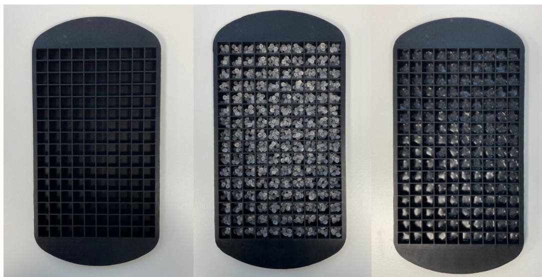
Figure 3 PP pretreatment by melting the pellets in silicon moulds into cuboids at 180 °C
