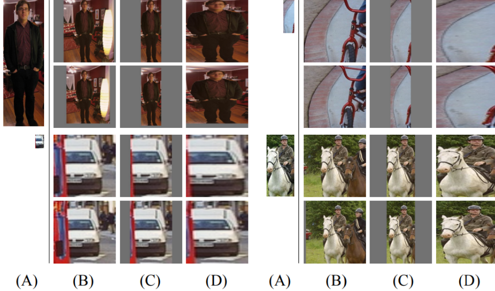
Figure 16: Different strategies for transforming the arbitrary shaped regions to have required size for the CNN input (227x227 pixels)[6]
