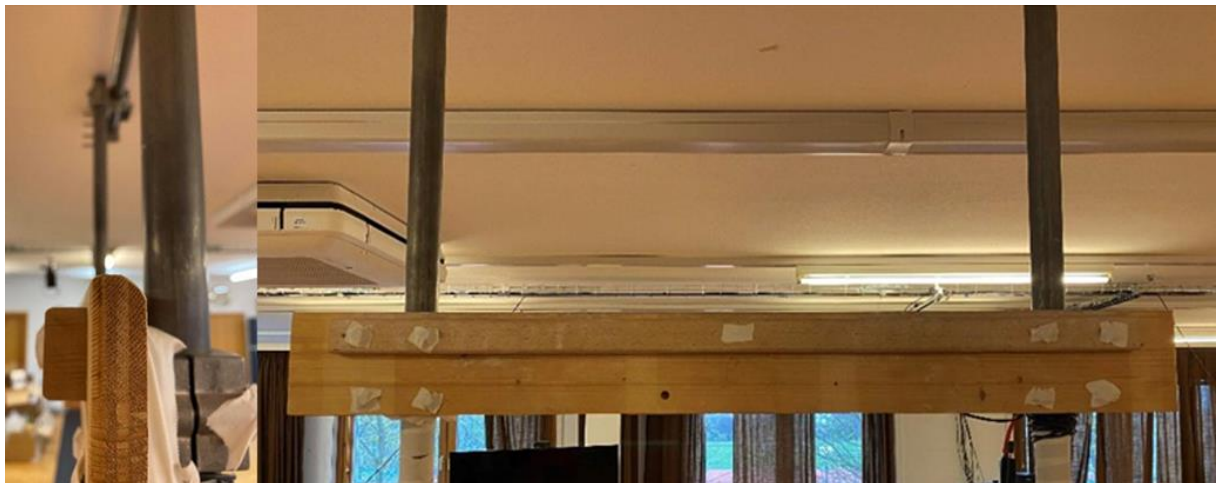
Figure 6: Self-made stable hangboard, attached to the ceiling with metal pipes (20 mm grip depth).
