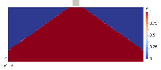
Figure 4.11.: Optimized topology for the realistic permanent magnet with \chi = 0.2 obtained with the objective functional defined in equation (4.22). The cells different with respect to the optimal topology obtained for \chi = 0 are colored in pink.
