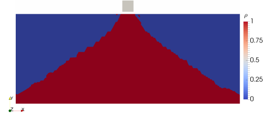
Figure 4.26.: Best optimized topology obtained using the RBTO algorithm for \chi = 10^2 , \rho_{\text{init}} = 0.5 , p = 1 and \eta = 0.01 .
