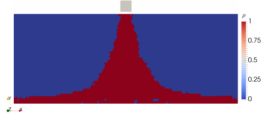
Figure 4.22.: Best optimized topology obtained using the RBTO algorithm for \chi = 10^3 , \rho_{\text{init}} = 0.5 , p = 5 and \eta = 0.01 .
