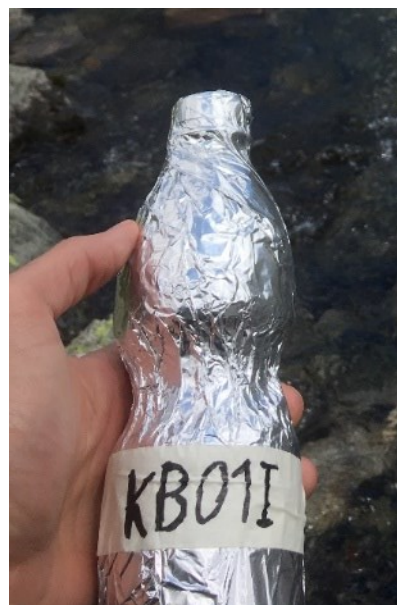
Fig. 13: Freshly wrapped 500 ml water sample for ^{129}\text{I} -measurement in the field
