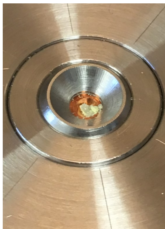
Fig. 18: AgI-powder on top of a copper target prior to being pressed with a piston
