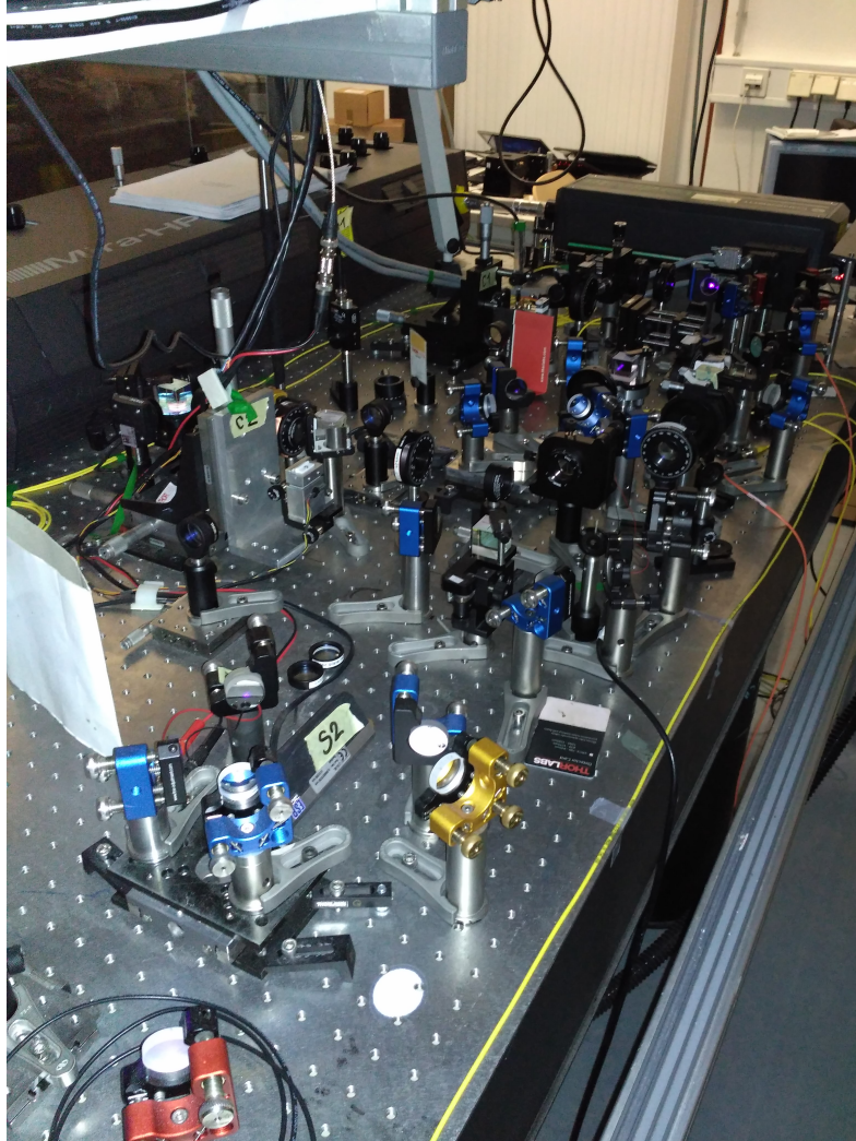
Figure 4.7: The photo of the actual experimental setup. The blue pumping laser beam enters the setup at the far end of the optical table. The holders of the first and the second non-linear crystals labeled by C1 and C2, respectively, are visible in the upper half of the image. In the foreground, the trombone system for the coarse adjustment of the phase in the second interferometer is visible.
