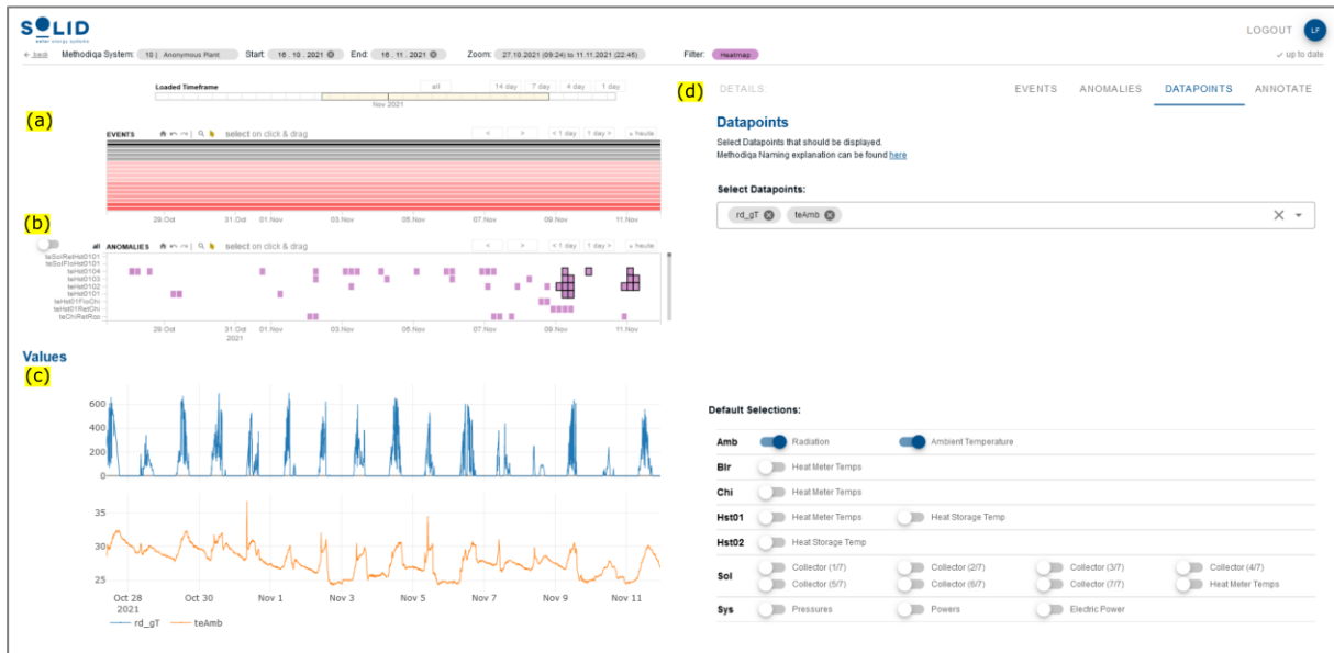
Figure 1: This work introduces the visual framework SunScreen, which supports Fault Detection and Diagnosis for solar thermal systems. It consists of four main parts: (a) shows manually annotated system events (e.g., services or faults) as a Gantt chart. (b) shows detected anomalies for each sensor as a heatmap, and (c) shows selected measurement values as a time series. Users can access more details about data points, events, anomalies, and annotations in the Details Panel (d).
