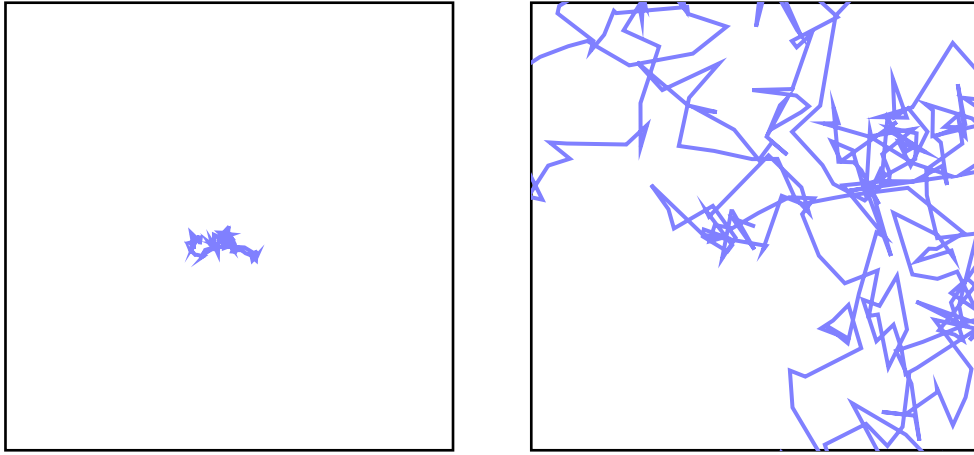
Figure 3.1: Schematic illustration of configuration space and the random walk. Our goal is to generate big steps (right) to reduce the number of steps needed before we can obtain meaningful data. Each point represents a measurement of the system in this state. We can emulate big step sizes by taking multiple steps in between measurements. This is especially important for calculations where we want to keep the number of measurements low, e.g. to visualize error bars.
